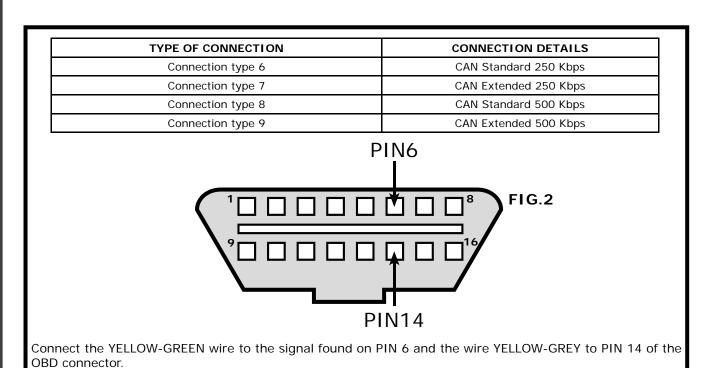
ATTENTION: The GREEN wire must be isolated and not connected
