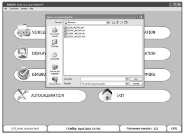
**NOTE:** To avoid losing the configuration of the control unit, make sure that the control unit is connected to the computer before updating. Whether or not the control unit is connected is indicated on the bottom left-hand side of the main menu screen.
