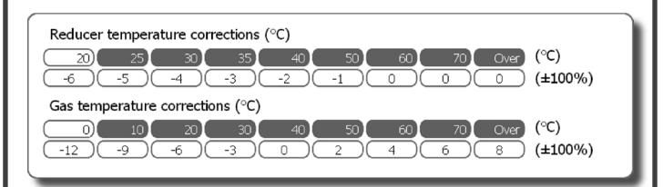
In this menu you can set percentage corrections on the GAS injection time obtained according to the temperatures of the reduction gear and of the GAS.
