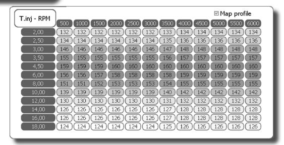
This menu shows a numerical display of the multiplication coefficients called K the control unit uses in calculating the GAS injection time.
