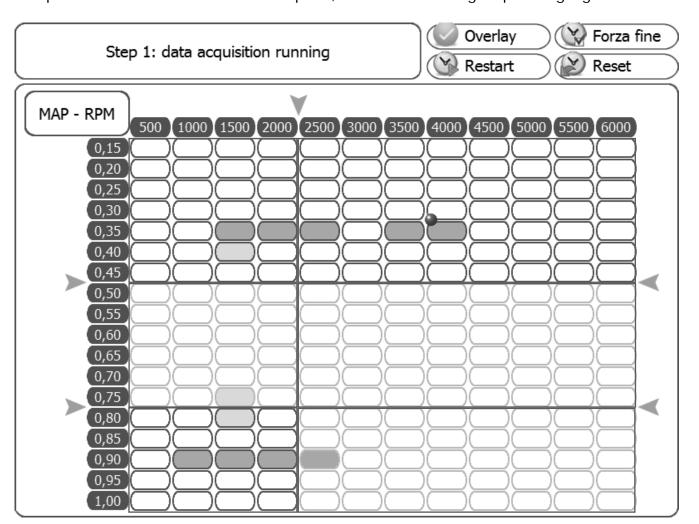
ATTENTION: If, for any reason whatsoever, the control unit is unable to acquire all the parameters required to calibrate the vehicle correctly, it will automatically switch to GAS after 3 hours and will start the acquisition phase while running on GAS.
