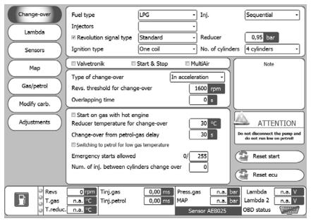
In the part underneath all of pages, a display summarising the current values of the general system operation signals is provided.
