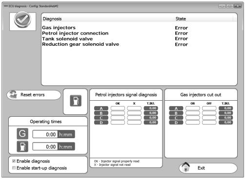
When the GAS control unit detects a diagnosis error on the parameter read, it will perform the action corresponding to the error detected. The possible diagnoses of the PETROL control unit are:
